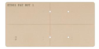
Minimum Body thickness for an F&T install is 1 3/4" (4,45 cm).
