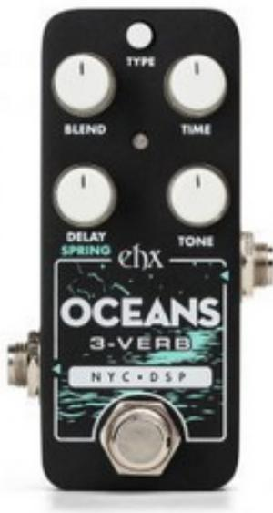
The EHX Pico Oceans 3-Verb is an ultra-compact reverb pedal packed with the essentials of ambience with plenty of flexibility and control. This Pico-sized reverberator adds the huge sounds of Spring, Plate, and Hall reverb to any pedalboard while using minimal space. Adjustable decay time, pre-delay / spring length, and tone make the Oceans 3-verb able to create a plethora of spacious sounds.
